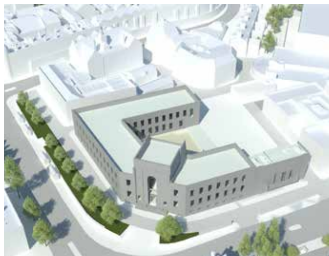
Potential scope of site clearance showing a possible extent of building removal whilst protecting and retaining the key external range of buildings, with their entrances and stairs.
